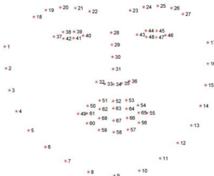
Fig.2. Visualizing the 68 facial landmark points
